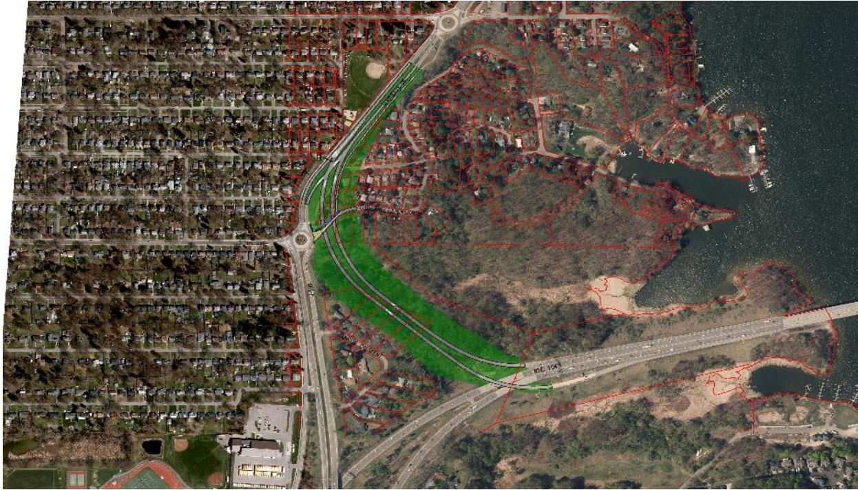
Figure 4-4 – Conceptual Layout of New Ramps at Irondequoit Bay Bridge
