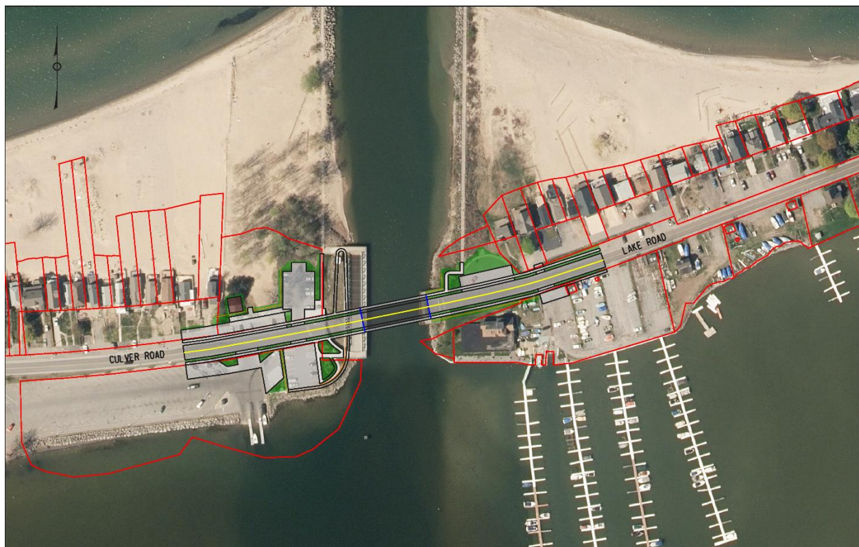
Figure 4-3 - Conceptual Layout of Retrofitting the Existing Bridge or a New Movable Bridge
