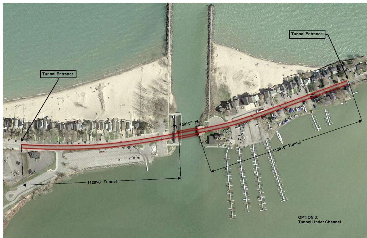
Figure 4-2 – Conceptual Layout of a Tunnel
