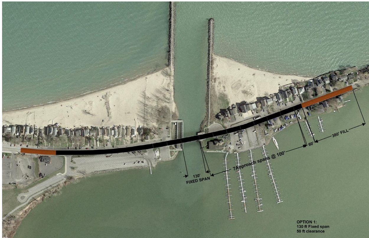
Figure 4-1 - Conceptual Layout of a Fixed Bridge with a 50-Foot Under Clearance
